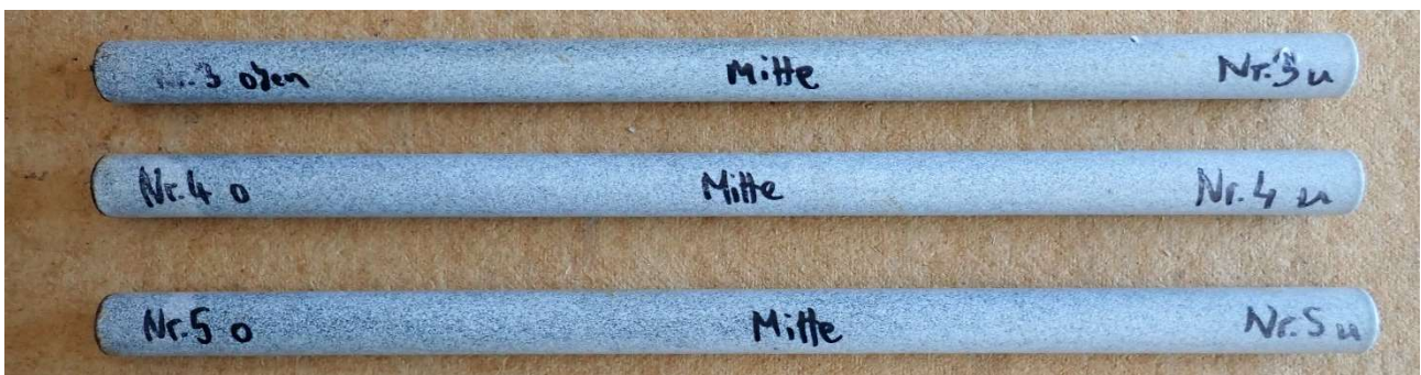
Picture 4: Opposite plastic coated surface of dowels without any rust in regarded area of lateral surface after 240 hours at neutral salt-spray.
