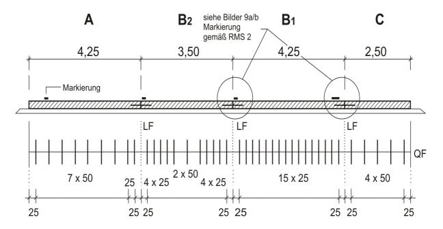
Tiebars are normally 20 mm in diameter and 800 mm long. The middle section (joint) of the tie bar is also coated with a ca. 0.3 mm thick plastic coating over a length of 200 mm to protect against corrosion.
