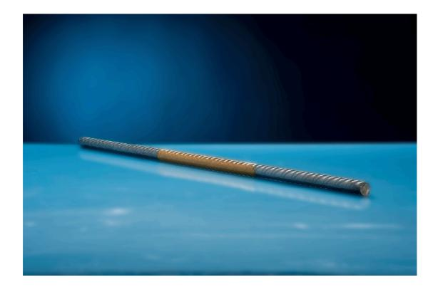
Our range of products includes plastic coated tiebars Ø 14 mm to Ø 28 mm in diameter and from 700 mm to 1200 mm long. The tiebars are conform to EN 13877-1 and are quality monitored by Munich Technical University, Institute of Road, Railway and Airfield Construction.
