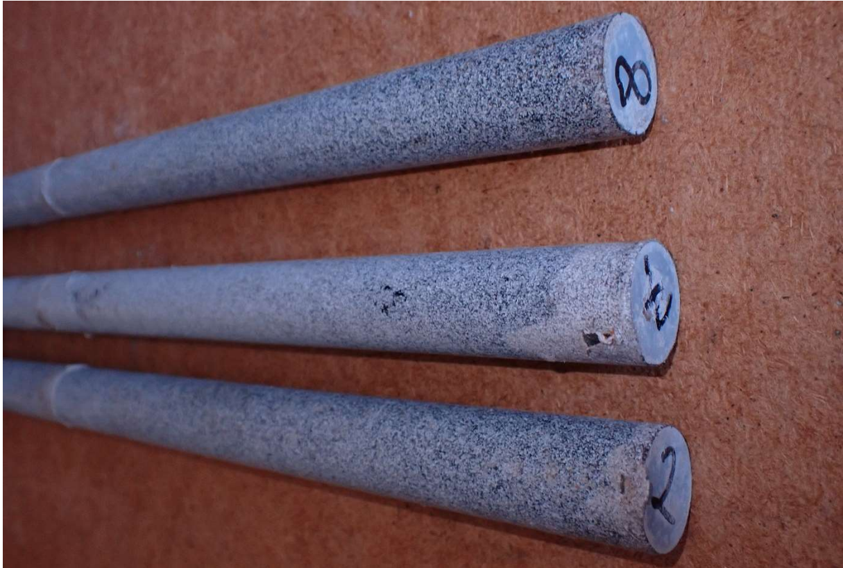
Picture 1: Tested dowels No. 2, No. 7 and No. 8 with delamination of coating at dowel No. 2 und No. 7 at the ending of the dowel.
