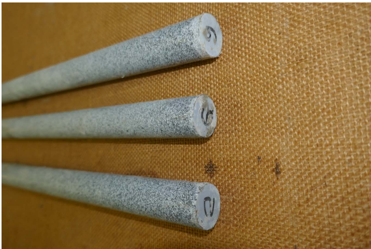
Picture 1: Tested dowels No. 2, No. 6 and No. 9 without damage or delamination of coating.
