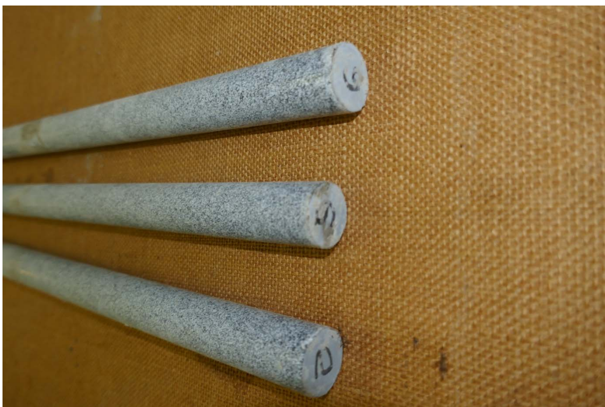
Picture 2: View of opposite side of lateral surface of dowels after test execution without damage of coating.
