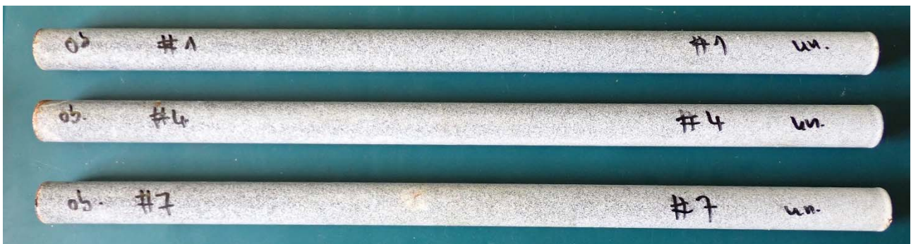
Picture 3: Plastic coated surface of dowels does not show any rust in regarded area of lateral surface after 240 hours at neutral salt-spray.
